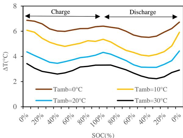
Figure 4. Effect of temperature on 60Ah battery temperature rise.
