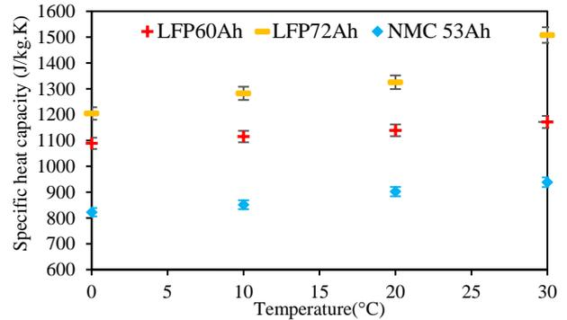
Figure 8. Measured specific heat capacity versus temperature.
