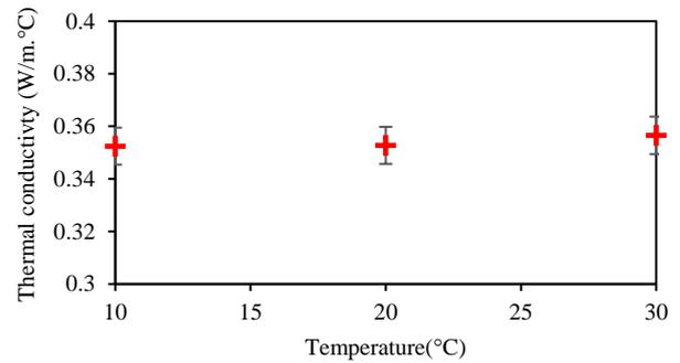
Figure 9. Measured thermal conductivity of the 60Ah LFP battery.
