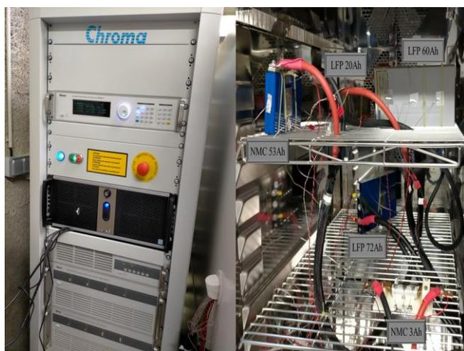
Figure 1. Experimental setup and tested batteries inside the climate chamber
